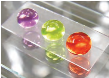
Transparent, superomniphobic micro-fabricated surface to repel all liquids.
