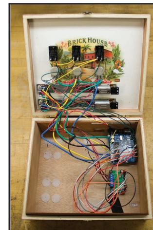
Inside the box are 3 switches, 3 rotary knobs, and 2 motorized faders. An Arduino microprocessor can be connected to a computer program like MATLAB, allowing simultaneous visual display of the virtual environment on a computer screen.
