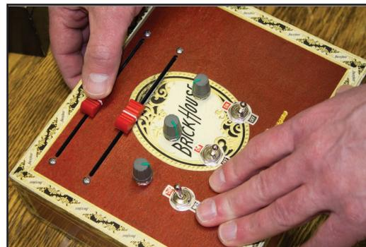
The red, motorized fader knobs allow students to feel and explore mechanical behaviors that change as they vary system parameters by turning the potentiometer knobs.
