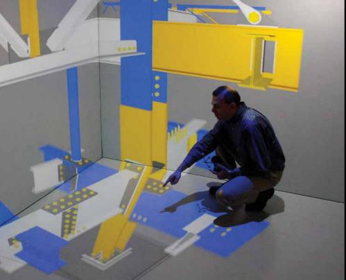
Digitized version of the steel sculpture lets students remove components, allowing a clearer picture of connections to emerge. The ability to reconfigure at will is a key advantage over the physical
