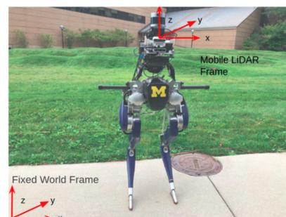
The Cassie bipedal robot provided measurements for Project #1 Map Building from LiDAR Data.
